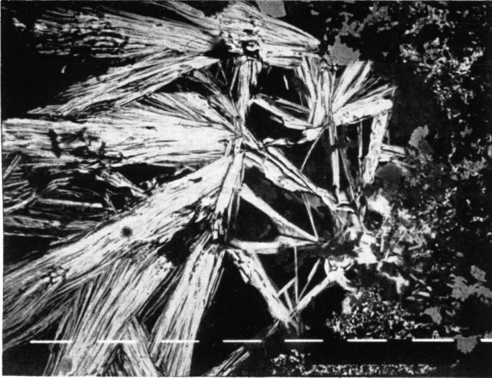
Fig. 2. The back-scattered electron image of cymrite. A bar indicates 10 \mu\text{m} .
