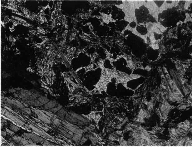
Fig. 3. Photomicrograph of pyrite grains surrounded by chamosite and calcite. One polar. Field view 1.3 \times 1.9 mm.
