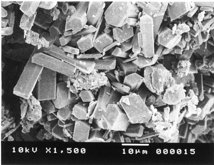
Fig. 2. SEM photograph of the aggregate composed of diadochite (prismatic crystals) and possibly kaoline minerals (platy crystals).
