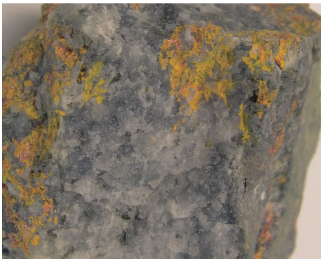
Fig. 1. Mixture of pararealgar and alacranite (both are yellow) inverted from realgar (orange) in quartz vein (NSM-M30973). Field view: approximately 4 \times 5 cm.
