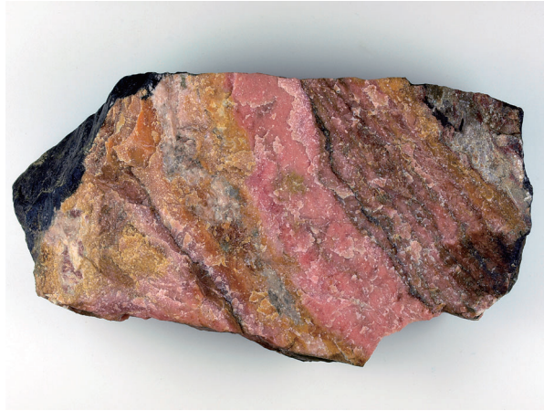
Fig. 1. The banded structure of natronambulite (orange), rhodonite (pink) and quartz (white). Specimen is approximately 12 cm wide.
