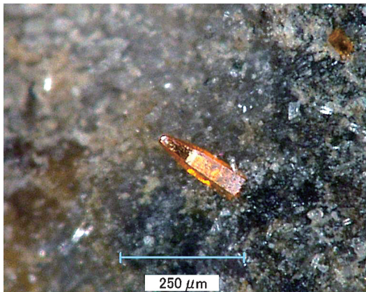
Fig. 2. Photomicrograph of rambergite crystal.
