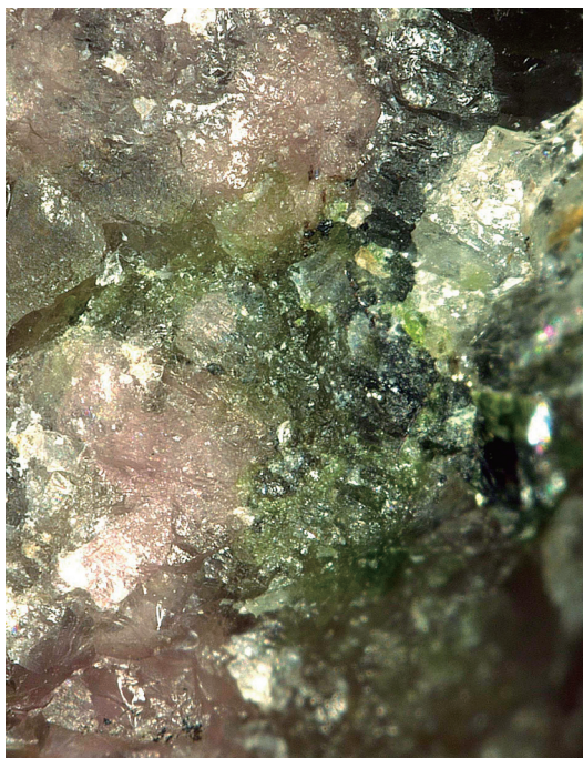
Fig. 1. Microphotograph of the aggregate of V-rich garnet including momoiite. Field view: approximately 2.9 \times 4.8 mm.
