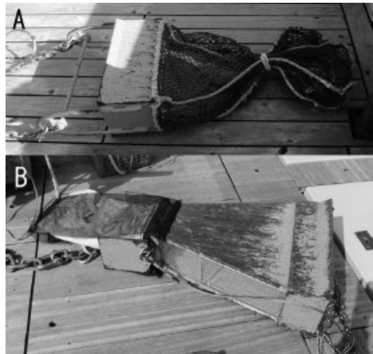
Fig. 2. Sampling gears; A, ORI biological dredge (50cm in width); B, modified Niino style dredge (50cm in width).
