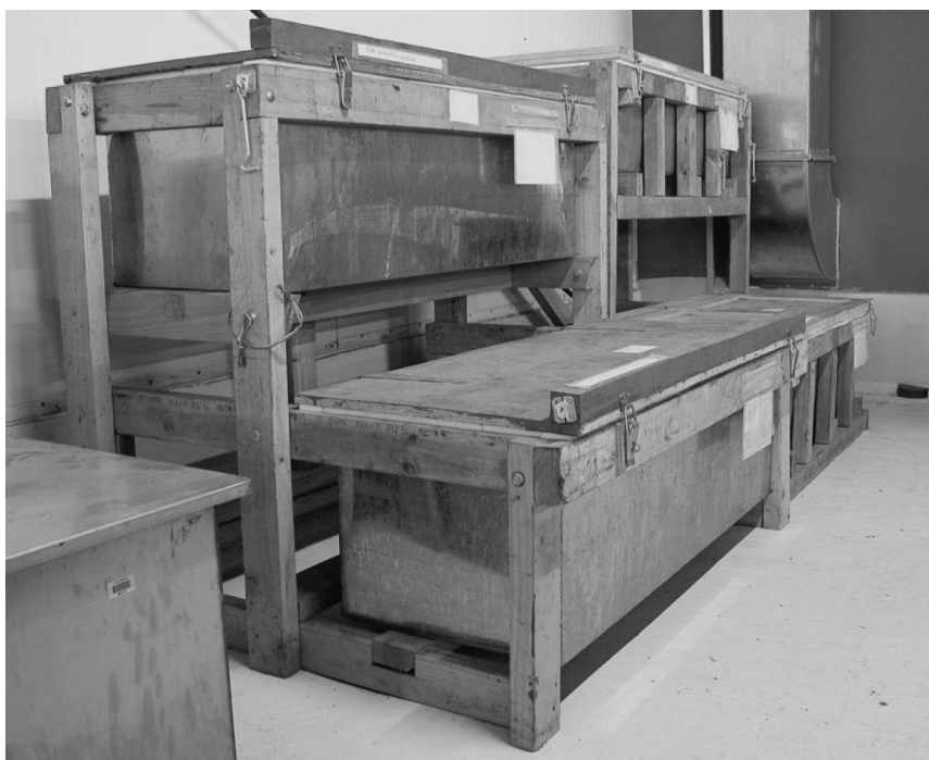
Fig. 3. Two medium sized (200 litre) stainless steel storage tanks set in a wooden frame to minimize space use while allowing access to both. (Photo: W. R. Webber)
