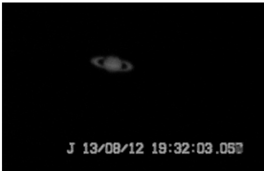
Fig. 2. Video image in which GPS time is inserted by GHS-OSD.
